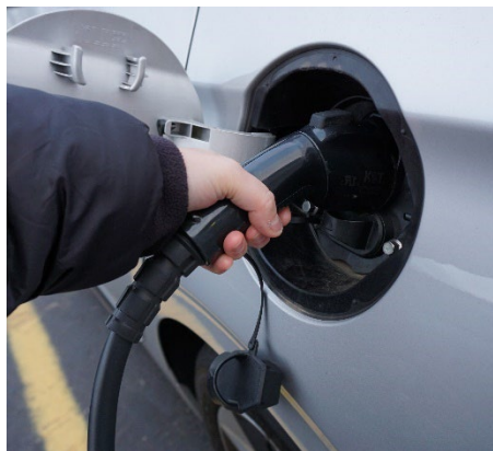
Connect the Charging Plug to the Vehicle
